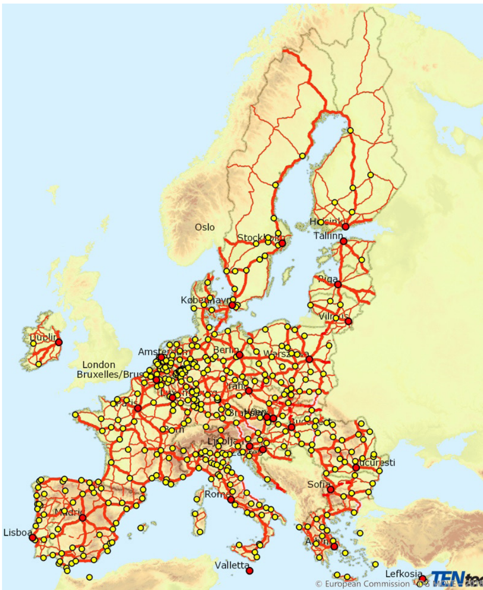
Figure 1. Map of the TEN-T network (European Commission, 2021a). Core and non-core network are shown in thick and thin lines, respectively. Yellow dots represent urban nodes. Red dots represent capital cities.
