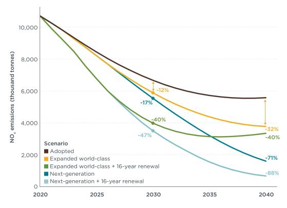
**Figure 5.** Diesel HDV exhaust  $NO_x$  emissions from 2020 to 2040 in G20 economies. Data labels show the percent change in  $NO_x$  emissions compared with adopted policies in 2030 and 2040.
