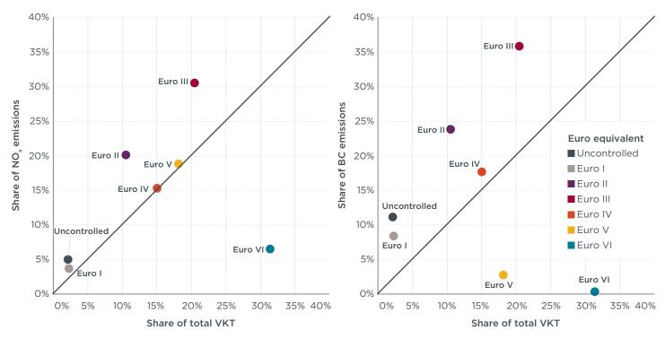
**Figure 4.** Share of total VKT (x-axis) and pollutant emissions (y-axis) by Euro-equivalent emissions standard, 2020. Points above the diagonal line indicate that vehicles of this standard have an outsized impact on emissions relative to their vehicle activity.
