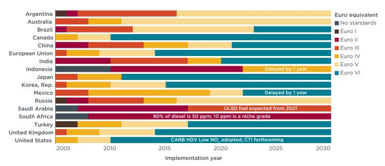
**Figure 1.** Implementation year (all sales and registration) of heavy-duty diesel engine emission standards in G20 economies. (France, Germany, and Italy, which hold separate G20 memberships, are included in the EU data.)
