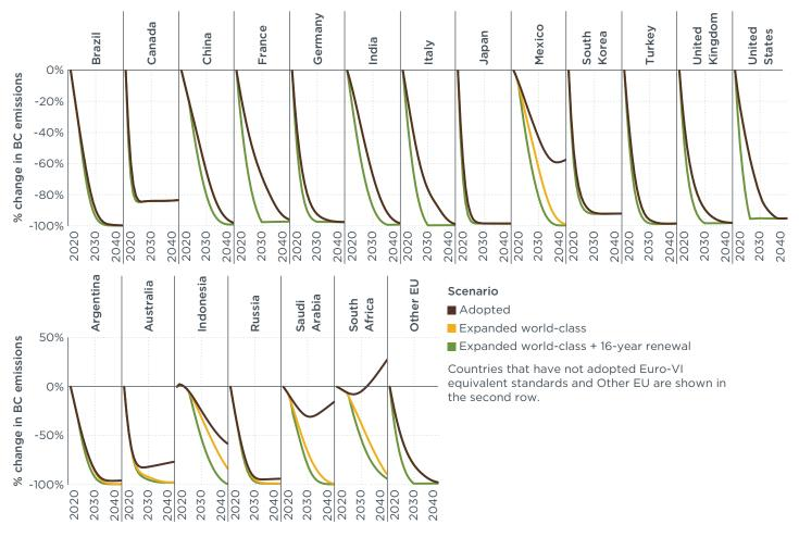
**Figure 8.** Normalized diesel HDV exhaust BC emissions from 2020 to 2040 by G20 economy. The y-axis shows the percent change in BC emissions from 2020.
