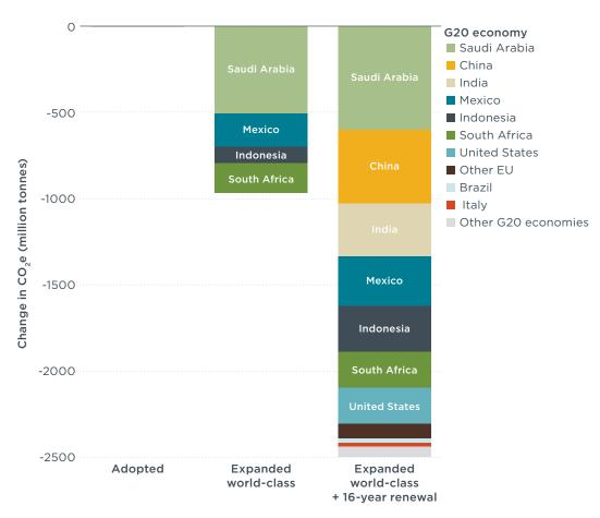
**Figure 17.** Cumulative mitigation potential (GWP20) for diesel HDVs under new policy scenarios compared with adopted policies, 2020–2040, ordered by mitigation potential in the next-generation plus 16-year renewal scenario.
