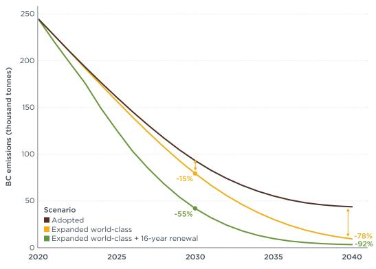
**Figure 6.** Diesel HDV exhaust BC emissions from 2020 to 2040 in G20 economies. Data labels show the percent change in BC emissions compared with adopted policies in 2030 and 2040.
